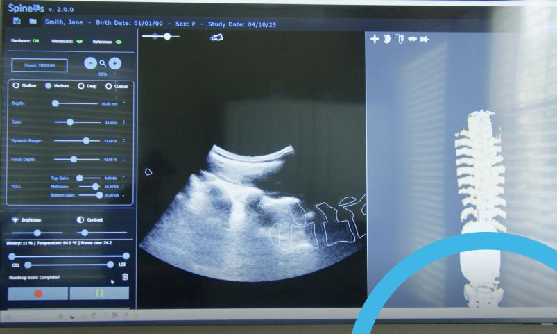
The SpineUs software application installed on the PC interacts with both OptiTrack's Motive motion capture software and the ultrasound scanner's firmware. By assigning tracking data to each captured ultrasound image, the software effectively synchronizes the ultrasound imaging data with the tracking data obtained through Motive.
